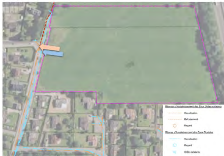
Raccordement assainissement – Cube²
