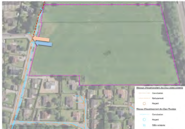
Raccordement assainissement – Cube²
